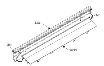
**Step 4:** Remove the tab at the top of the Shield from the slot in the Base Channel.
